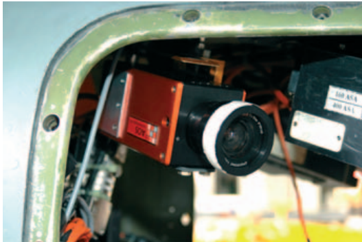
X-EMA positioned inside pod
