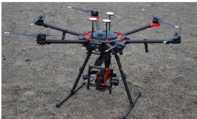
L-BLAST mounted on drone and ready to fly
